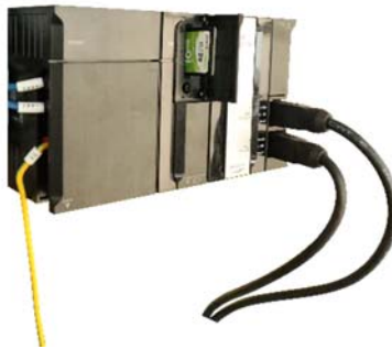
Figure 7-48 SD card slot position
